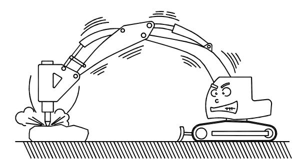
[2] On the contrary, when position is excessive enough to break rocks with front of the base machine raised, the machine may suddenly tilt forward the moment rocks are broken. Then, the breaker body or the end of bracket may violently hit against rocks and result in damage.
