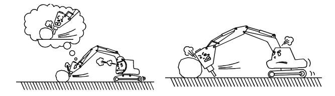
[6] Do not use rod as a lever. Do not put the rod into a crack in rock and move the rod to and fro to breaker the rock, otherwise the rod will be broken or the bracket will be damaged.
