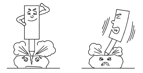
[4] Apply same direction of boom force in line with the rod and place the rod in the rock with hammering surface as vertical as possible. If hammering surface is oblique, the rod may slip during hammering. This causes the rod to seize and to be broken and piston to be damaged. When breaking, fully stabilize the rod first and then select the point of a rock on which hammering can be performed in a stable condition.
