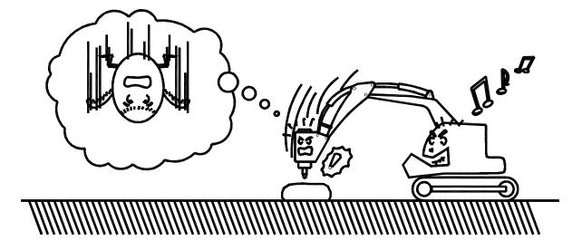
[9] Breaking operation conducted at the stroke end(when the cylinder is extended or retracted to a maximum extent) of respective hydraulic cylinders of the carrier will lead to damage to the cylinders and other parts of the carrier.
