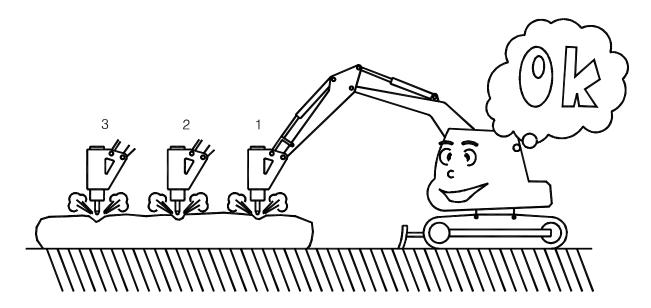
[5] Rolling or falling a rock with the rod end or bracket side by using the boom or arm of the carrier as shown in the figure will result in breakage of the breaker mounting bolt or bracket, breakage and galling of rod, and damage to the arm and boom. Do not move rock. It is strictly prohibited to travel when the breaker is in the contact with rock.
