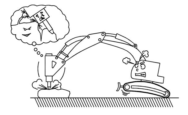
[3] It is undesirable to carry out hammering under the below condition, because vibrations during hammering may be transmitted to tracks of the base machine.
