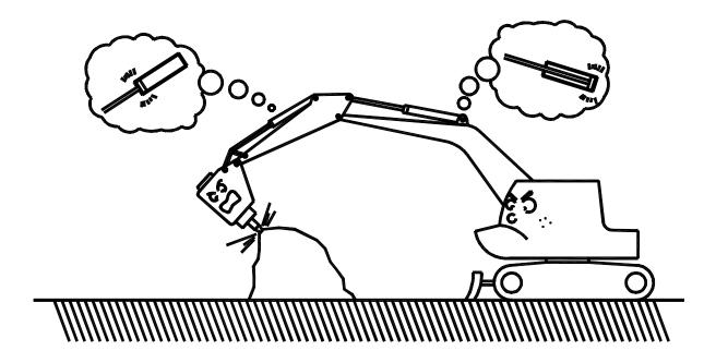
[10] Lifting thing by hanging wire in the bracket or rod not only causes damage to the breaker but also is very dangerous.
