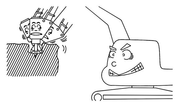
[7] Do not operate breaker when all components except rod are immersed in water and mud. Underwater usage of the breaker will cause internal damage to the breaker. Consult Soosan for modifications if you have an underwater requirement.
